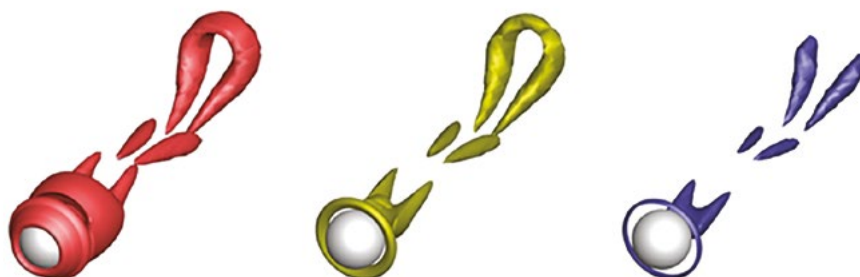
Figure 2. Vortices identified by Q , Q_w and Q_M (isovalue 0.1). The criterion Q_w is optimal, see [6] for details.
