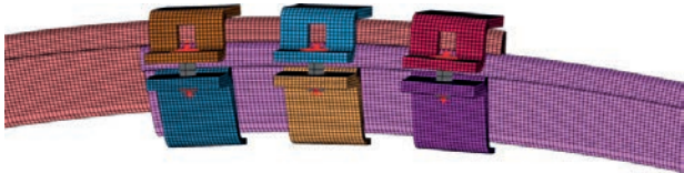
Figure 1. FEM model of yielding connection
